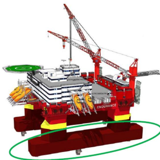
Figure 2: Pontoons of the Vessel (circled in green)
