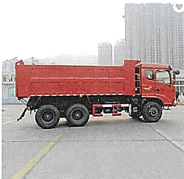
*Heavy Duty 15m cube load volume 20 ton[ne] tipper truck
